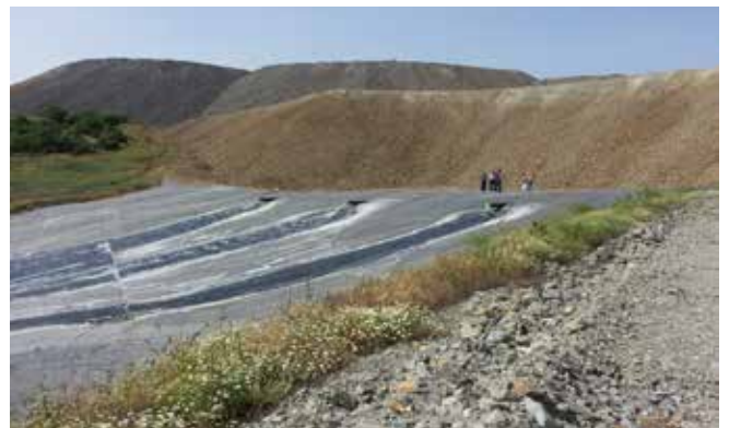
Fig. 4 - 5. The bioleaching of dumps of low-grade copper ores near Radovich, Macedonia
